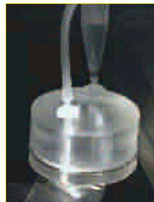
Introduction of the liquid containing magnetic nanospheres into a microchannel in a silicone rubber wafer. (Courtesy of the Institut Curie.)
